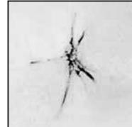
This break consists of a pit with radial cracks. The cracks do not penetrate through to the lamination. There is little or no air to displace, allowing a minimum of resin to penetrate. Results will vary
